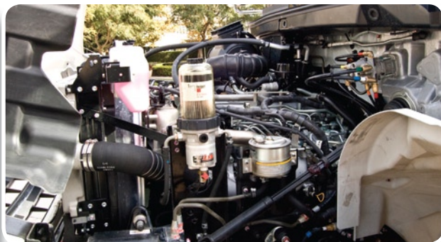
Engine compartment upgrades for the 2011-model 238 and 338 include a 130A alternator, more efficient turbo with an 11 curved vane design, and an improved combustion chamber design. Other redesigns include the fuel filter, now under the hood, and a more efficient single EGR cooler.
