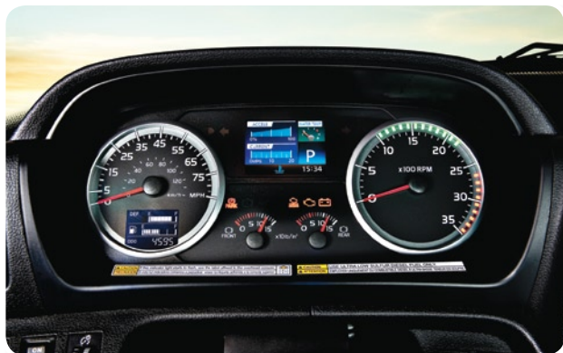
The new cluster also features a gauge for diesel exhaust fluid (DEF) level and an advanced audio alert/warning system informing drivers of low DEF levels.
