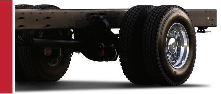
Hino Trucks' standard 80,000 PSI frame is among the strongest in the industry. An optional 120,000 PSI frame is available (L7 only) to maintain integrity in the most rugged applications.
